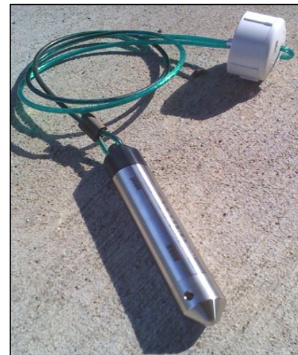
Figure 5. Probe used to measure water level and temperature in Beebe Lake (HOBO 13-ft water level probe, Onset Computer Corp.)
