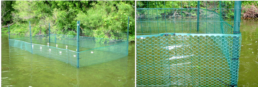
Figure 6. Installed fenced plot with PVC cell markers (left), and close-up of fencing (right)
