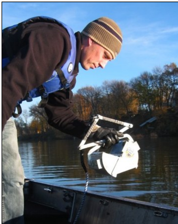
Figure 4. J. Johnson (Freshwater Scientific Services, LLC) collecting sediment samples with a petite Ponar grab sampler (left); sprouted curlyleaf pondweed turions (above)
