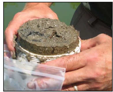
Figure 5. Sediment samplers used to monitor study lakes. Ponar dredge (left) and PVC suction corer with extension for flocculent sediment (right). Core sectioning (below) conducted by placing core tube onto a plunger stand, extruding the core contents, and removing sediment to the desired depth for each stratum.
