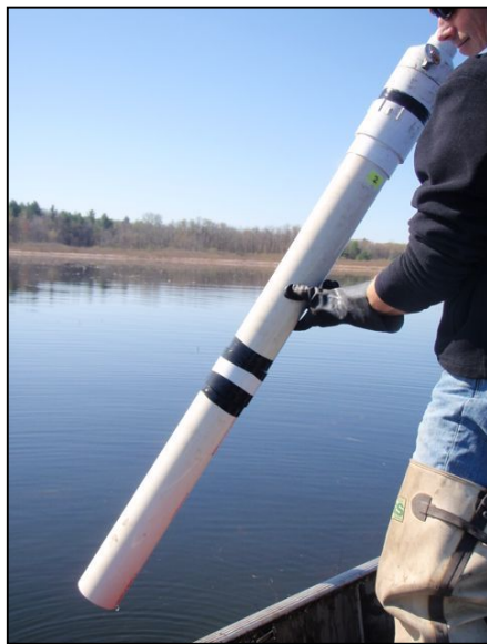
Figure 5. Sediment samplers used to monitor study lakes. Ponar dredge (left) and PVC suction corer with extension for flocculent sediment (right). Core sectioning (below) conducted by placing core tube onto a plunger stand, extruding the core contents, and removing sediment to the desired depth for each stratum.
